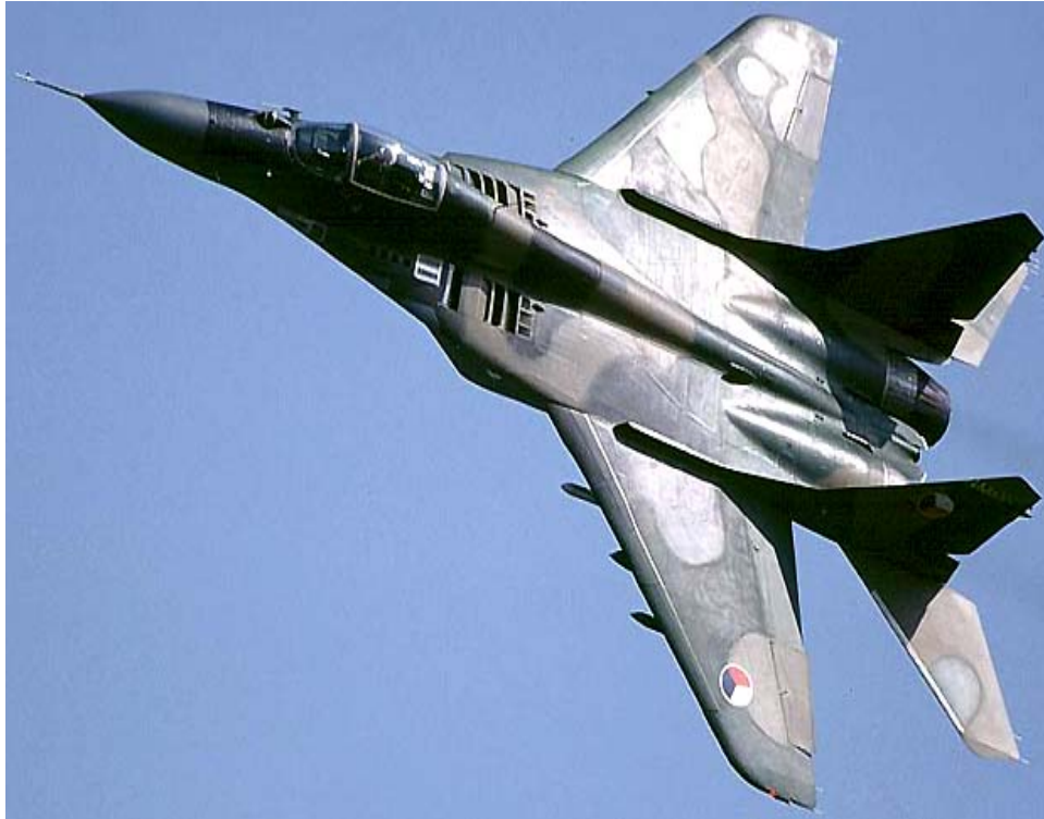
Fig.6.12 Airplane with two vertical tails MIG-29M (Adapted from: http://www.defenseindustrydaily.com )
