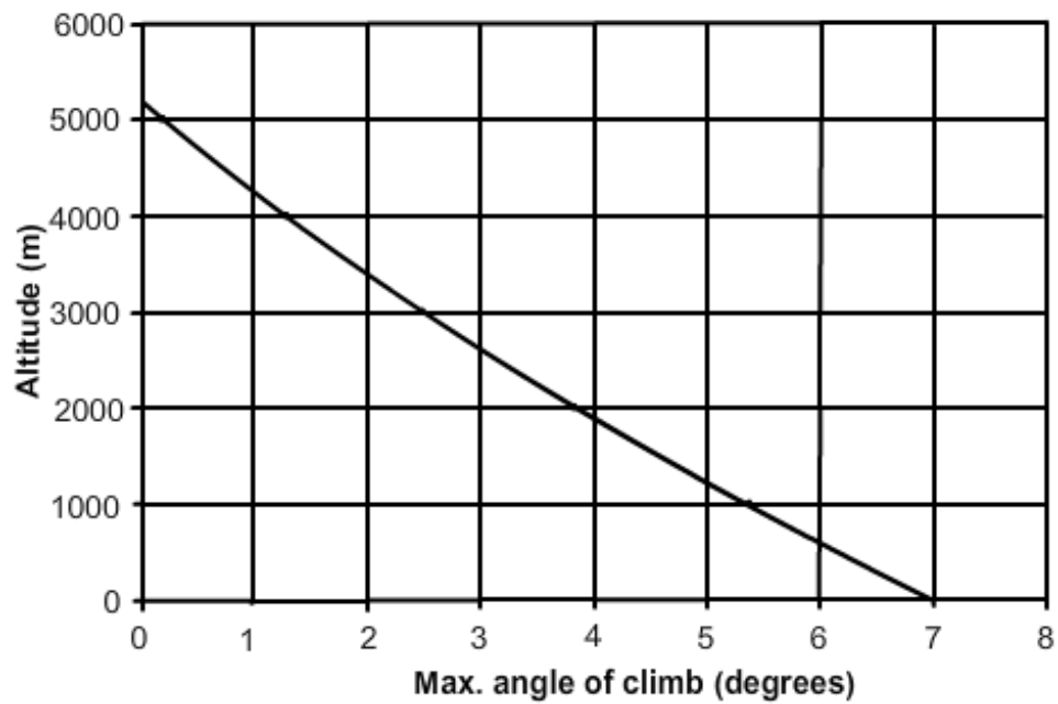
Fig.15 Variation of maximum angle of climb with altitude
